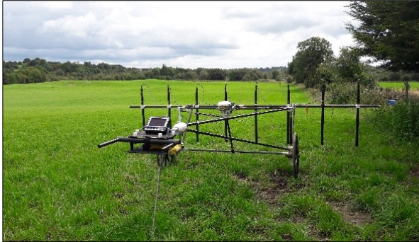
4. Advanced multi-channel gradiometer system for magnetometer survey (manual configuration).
